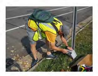
Figure 3.2: Setting up a traffic recorder
